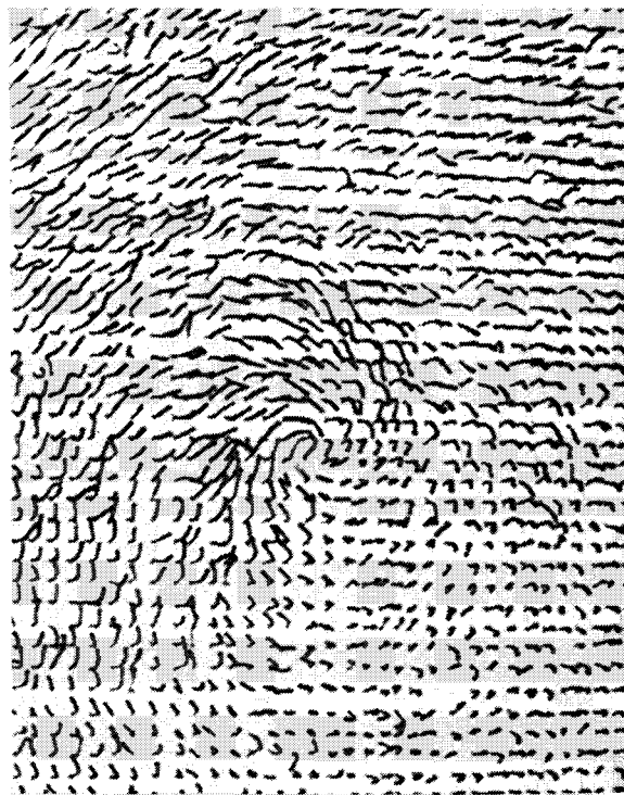
Fig. 2 Vortex shown by tuft grid.
